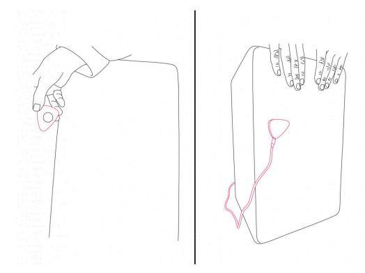
Remove the other side's protective later and firmly press the AP-1 on the desired place of the instrument.
