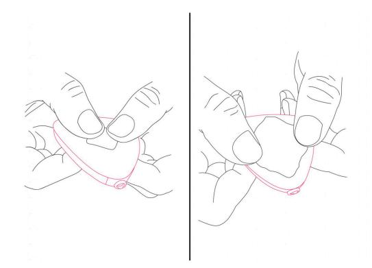
Take a small amount of putty and stretch it to a shape that will cover more of the bottom of the pickup. Place it in the middle of the pickup.
