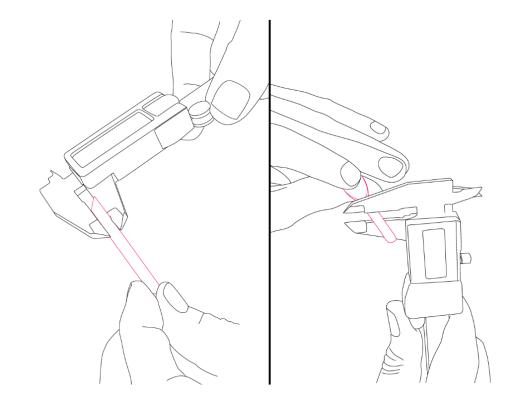
Using a caliper, measure the height of your saddle you have just removed.
