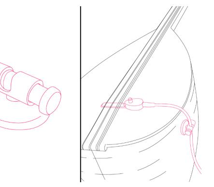
Choose the most convenient place to attach the provided KNA safety cable clip.
