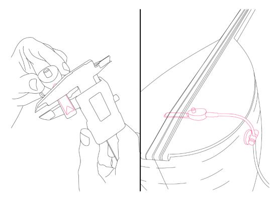
Once the proper height is achieved, use the provided double sided adhesive strip to attach the ebony saddle on top of the pickup.
