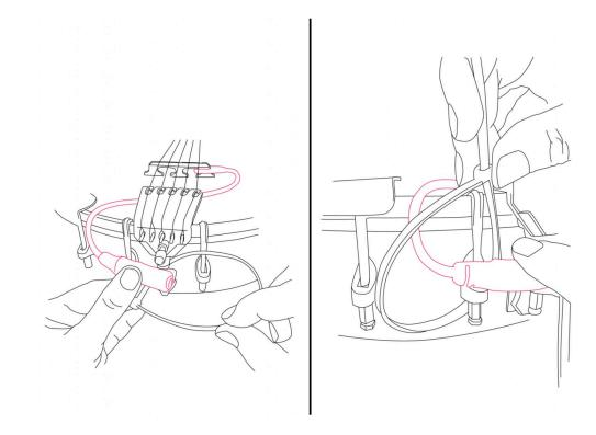
Find a suitable place for the jack housing near the tailpiece.
