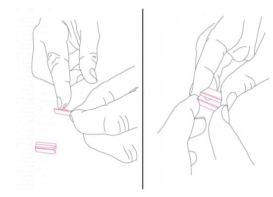
For narrower bridges, the provided shims may be required. Peel the protective film off and install on the flat side of the microporous sleeve. For your convenience, stick the shims on the microporous sleeve while it is removed from the sensor. For stable attachment, install as many shims as needed.
