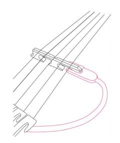
The sensor should stay stable on the bridge. If needed, you may move it toward the bottom of the bridge where the bridge is wider. Hold the sensor carefully with your fingers on both sides and carefully slide it down. The sensor should fit tightly but shouldn't require force to be placed in position.
