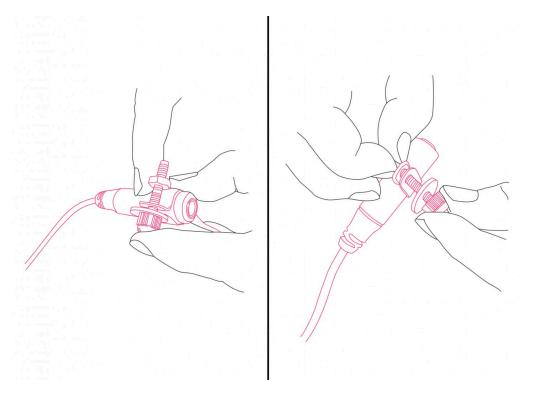
To attach the jack clip to the tailpieces, unscrew the nut and washer to completely open the retaining bracket with the clamp. Remove the washer.
