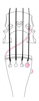
You can use a slotted screwdriver to tighten additionally if needed. Do not overtighten to avoid damaging the screw thread or tailpiece. Always hold the jack housing with one hand while plugging and unplugging the cable.
