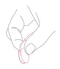
If the slot is wider than the sensor use the additional provided shims. Line up the necessary number of shims along with the sensor and slide them in the slot under the 1st (G) string. The sensor will operate equally well from either side of the bridge. We recommend installing the sensor on the right side of the bridge (G string side). Some players prefer to install the sensor on the left side (E string side).
