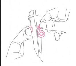
Feed the screw through this slot and the washer. Tighten the washer screw, holding the nut with the fingers of your other hand.
