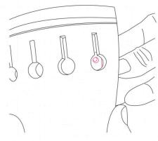
Position the retaining bracket beneath the tailpiece near the G string slot. We recommend installing the jack housing on the right side of the tailpiece (G string side).
