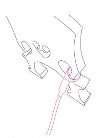
The sensor should be facing down with the flat side of the lead cable. Hold the bridge with one hand so it does not move while installing the sensor. The sensor should fit tightly but install without force. It should not move while playing or even shaking the double bass, but not too tight where the sensor or bridge can be damaged or broken.
