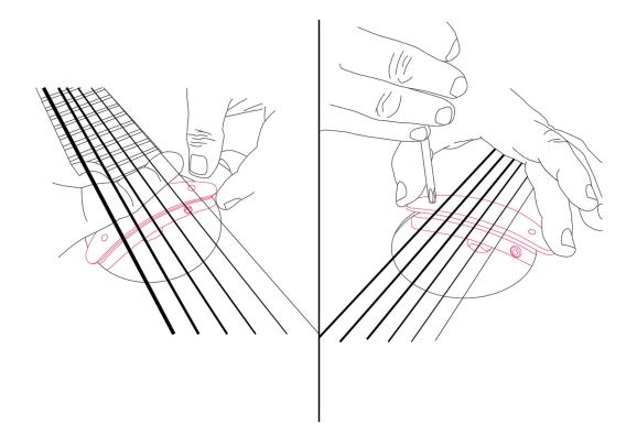
Position the pickup into the soundhole using the two side slots. Move up to the neck side, positioned below the end of the fingerboard. Using a Philips screwdriver, gently tighten the mounting screws until the pickup sits securely in the soundhole. Make sure not to over-tighten, as the screws can strip or the finish of the guitar could be damaged.
