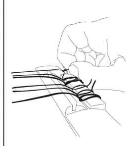
Loosen the strings of your guitar. Make sure there is enough space under the loops so the pickup can slide through without any pressure.
