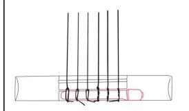
Slide the pickup under the string loops. Keep it positioned evenly on the tie bar while tightening the strings and retune.
