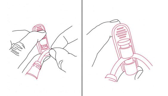
Press the top button to open the safety clip. Insert your instrument cable into the opening and release the button.
