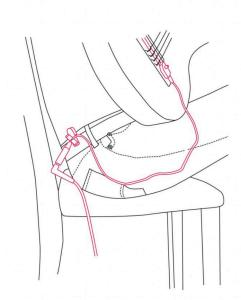
Hold the pickup head securely when attaching and detaching the cable.
