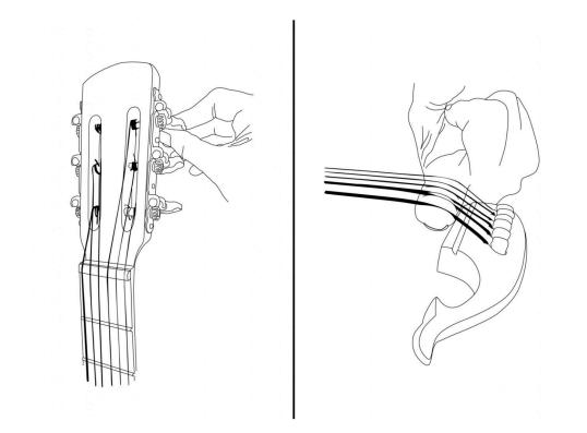
Loosen the strings of your guitar. The pickup will be inserted between the bridge pins and the saddle. The bridge saddle should have a minimum of 2.5mm (0.098") height on the treble side to allow room for pickup placement and for it to function properly.
