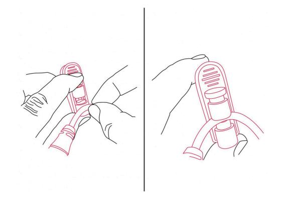
Press the top button to open the safety clip. Insert your instrument cable into the opening and release the button.
