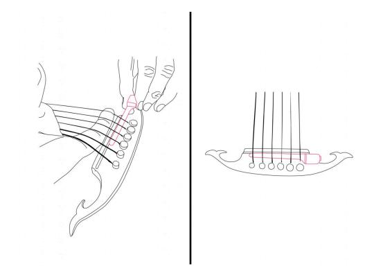
Starting with the narrow end, slide the pickup between the bridge pins and the saddle. Move the pickup from the treble side up to the bass side until the end rests below the last string.
