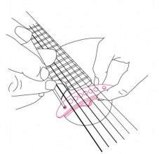
Position the pickup into the soundhole using the two side slots. Move up to the neck side, positioned below the end of the fingerboard. Using a Philips screwdriver, gently tighten the mounting screws until the pickup sits securely in the soundhole. Make sure not to over-tighten, as the screws can strip or the finish of the guitar could be damaged.
