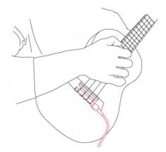
Hold the pickup head securely while attaching and detaching the cable.
