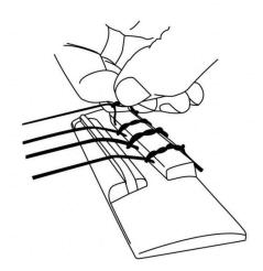
Loosen the strings of your ukulele. Make sure there is enough space under the loops so the pickup can slide through without any pressure.
