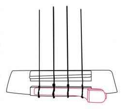
Slide the pickup under the loops. Position it evenly on the tie bar while tightening the strings and retune.
