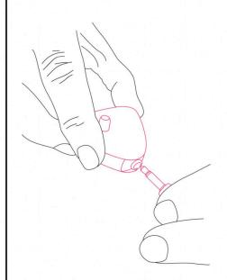
Place the pickup on a selected area of your instrument's soundboard. This may be the top of a guitar, or flat side of a drum.
