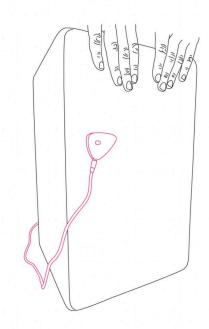
Remove the other side's protective later and firmly press the UP-2 on the desired place of the instrument.
