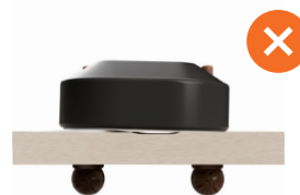
Fig 1.1 Sensor placed on uneven surface
