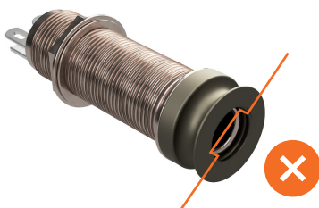
Fig 10.1 Jack tip NOT to be recessed inside strap-ring.
