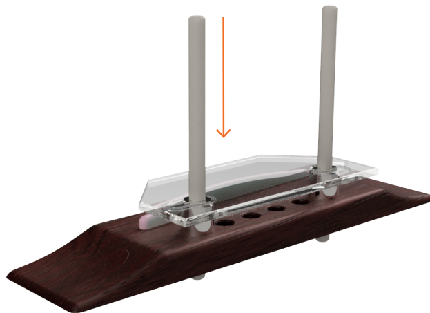
Fig 3 Lower mounting-jig on to bridge top.
