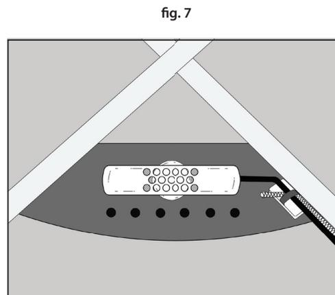
This is an internal view with the Tru • Mic mounted on the center of the bridge plate. The Tru • Mic and Element wires are secured with one wire clip on the bass-side of the bridge plate near the exit hole.
